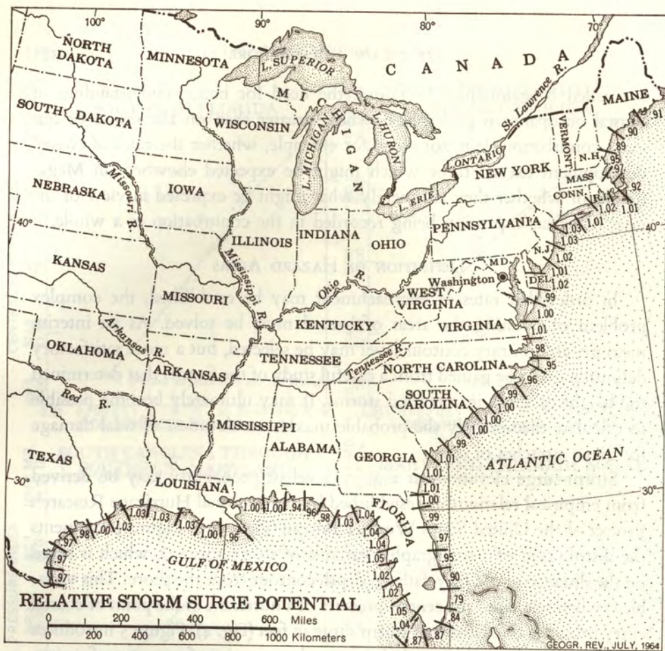
FIG. 3—Relative storm-surge potential of different coastal sections. Adapted from National Hurricane Research Project Rept. No. 32 , U. S. Weather Bureau, Washington, 1959, Fig. 4 (p. 8).
